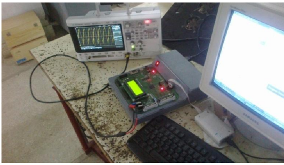
Fig.15. Experimental setup for downloading the design in SPARTAN6 FPGA
