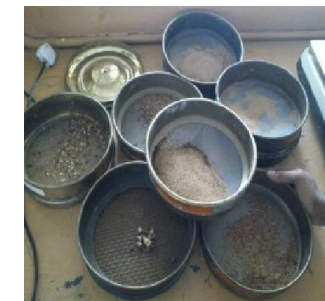
Fig.9. SIEVE method for calculation of the size of different particles in the soil sample
