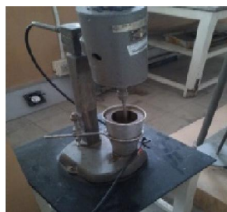
Fig.7. Soil samples being powdered for hydrometric test
