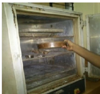
Fig.6. Soil samples being kept in the oven for VWC calculation
