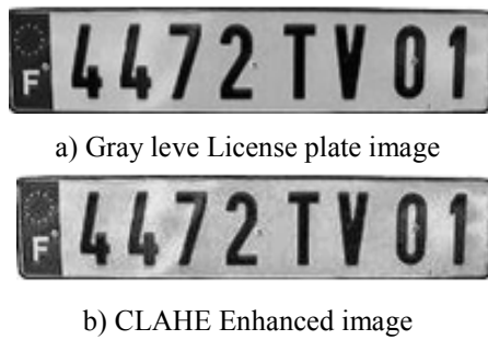
Figure 3. Example of CLAHE enhanced license plate WIENER FILTERING
