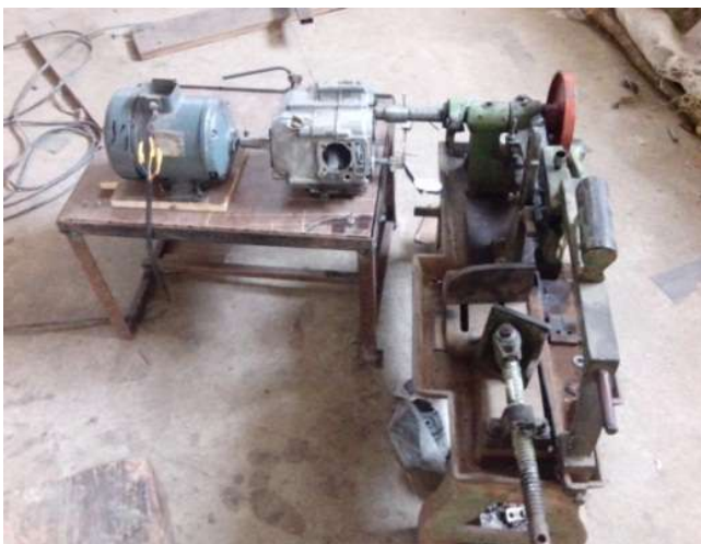
Fig. 2. Construction of Clutch Operated Gear Driven Power Hack Saw
