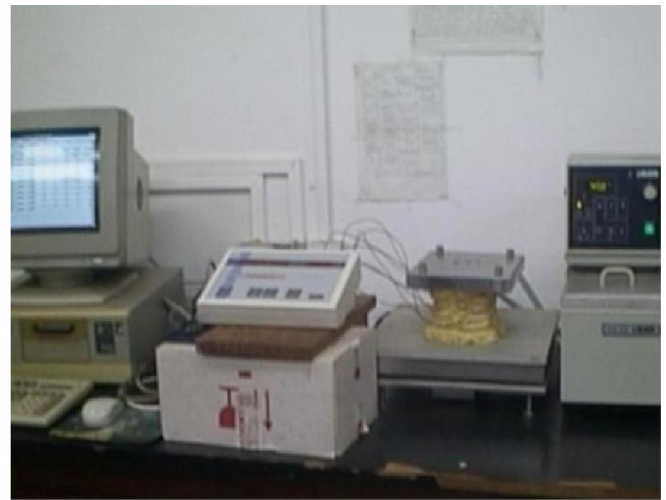
Fig. 1. The complete instrumentation of measurement of thermal conductivity by the comparison method (Allognon, 2007)
