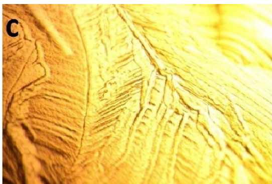
Figure 4. Crystallization of unpurified polysaccharide under light microscopy (a), Crystallization of purified polysaccharide under light microscope (b and c) which had regular and dense shape of crystal but unpurified polysaccharide had irregular and subtle shape of crystal
