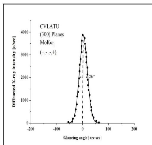
Fig. 6. HRXRD curve of CVLATU crystal
