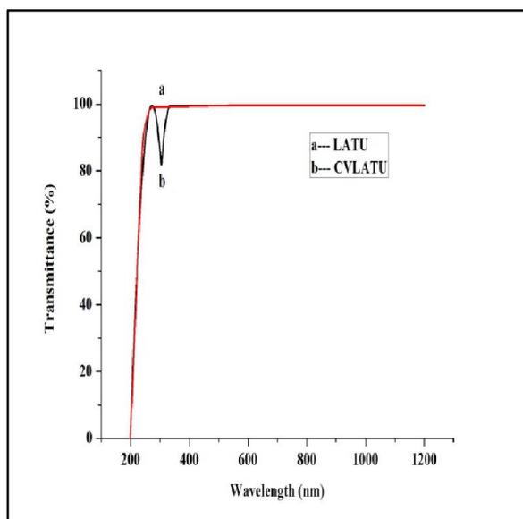
**Fig. 9. UV-vis-NIR absorption spectra for LATU and CVLATU crystals**
