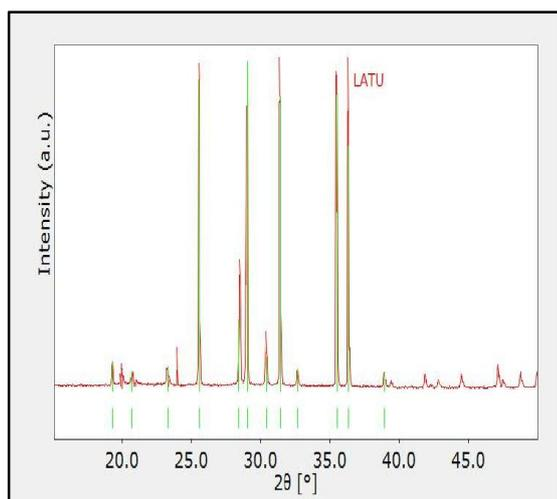
Fig. 3. PWXRD spectrum of LATU crystal
