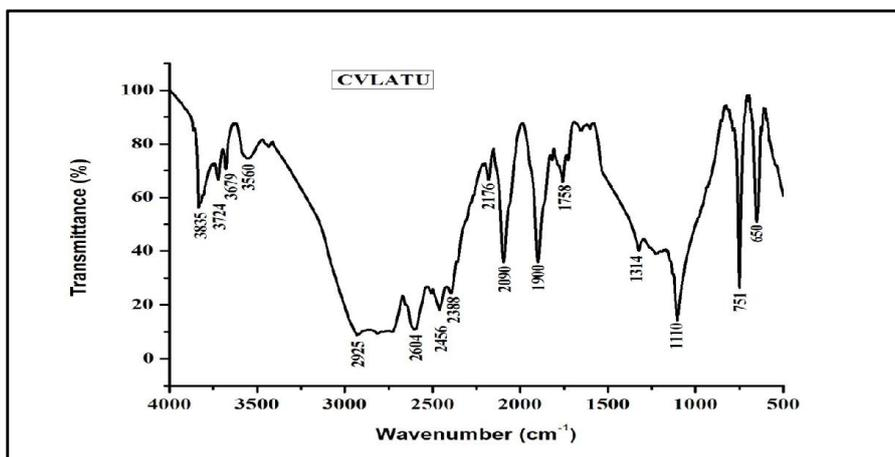
Fig. 8. FTIR spectrum of grown crystal violet dye admixed LATU (CVLATU) single crystal.
