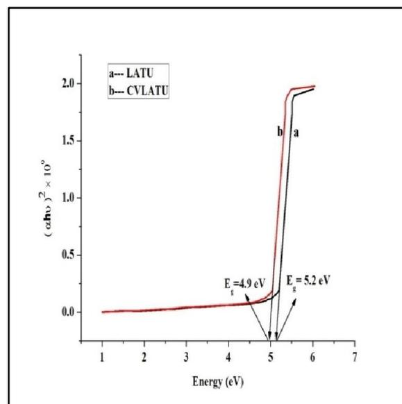
**Fig. 10. Photon energy vs  $(\alpha h\nu)^2$  for LATU and CVLATU crystals**
