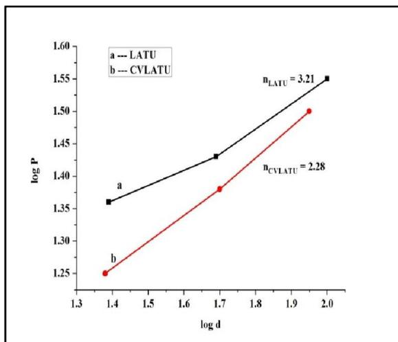
**Fig. 16. Variation of log (P) with log (d) for LATU and CVLATU single crystals**
