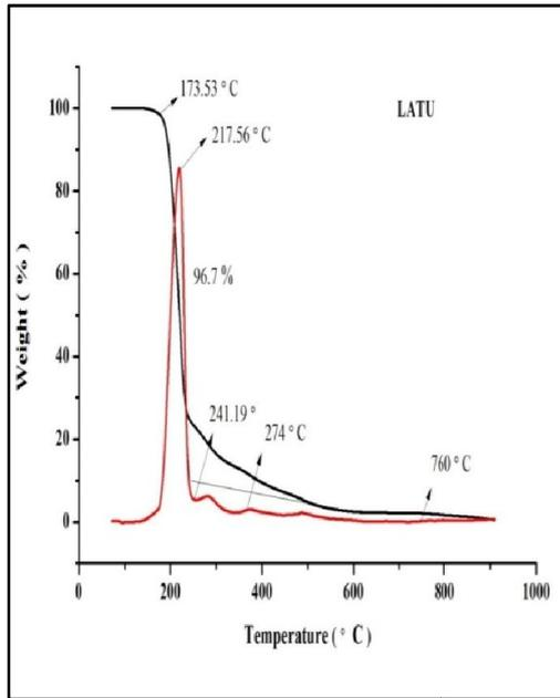
Fig. 11.TGA and DTA curves of LATU crystal
