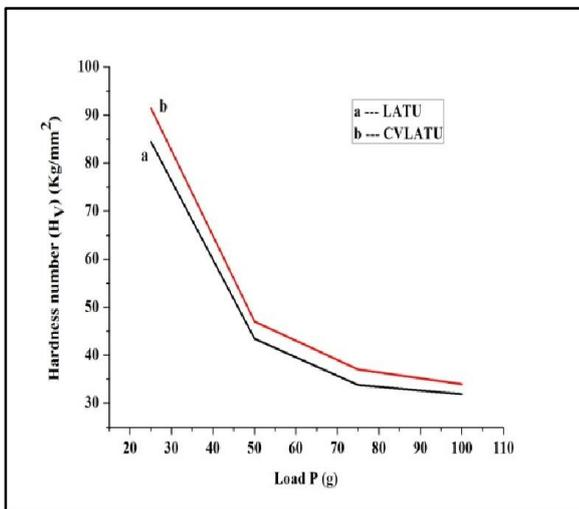
**Fig. 15. Variation of hardness with applied load for LATU and CVLATU single crystals**
