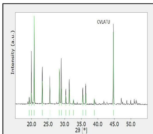
Fig. 4. PWXRD spectrum of CVLATU crystal
