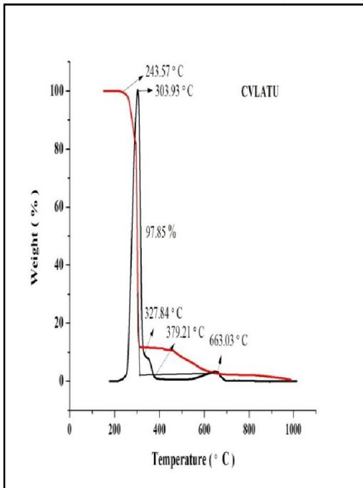
Fig. 12. TGA and DTA curves of CVLATU
