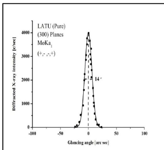
Fig. 5. HRXRD curve of pure LATU crystal
