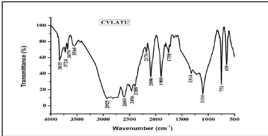
Fig. 8. FTIR spectrum of grown crystal violet dye admixed LATU (CVLATU) single crystal.
