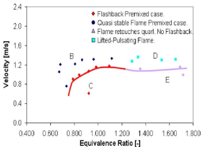
**Figure 18. Different regions in the flashback map at atmospheric conditions using the Quarl Nozzle with injector. B) region of quasi stability for the flame, various shapes. C) Flashback region. D) Lifted flame. E) The flame retouches the quarl**
