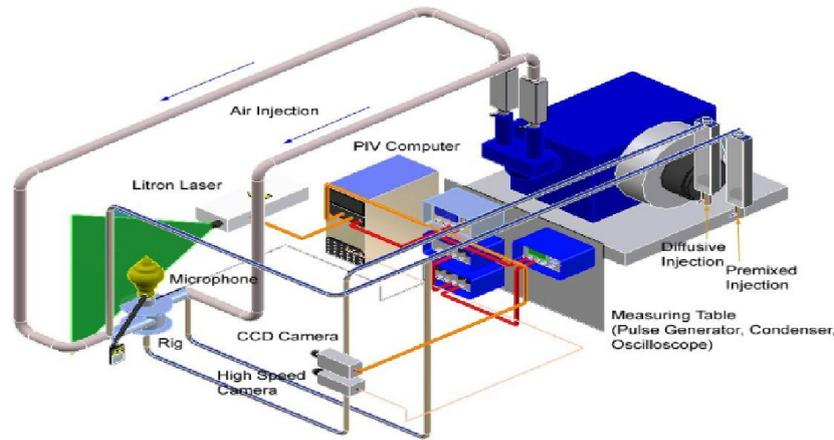
**Figure 2. Setup of the Entire System, including HSP and PIV, Fuel is injected via 2rotameters (yellow arrows) whilst air is tangentially introduced at different flow rates**
