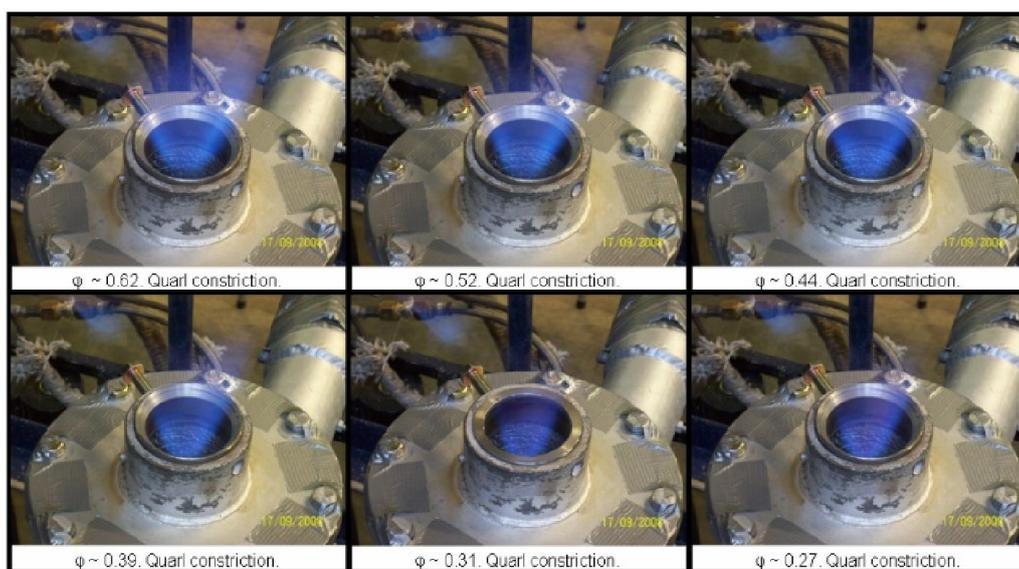
Figure 13. Quarl constricted case at different equivalence ratios. Gas Injection of 25 l/min diffusive (Wide Injector), 40l/min premixed
