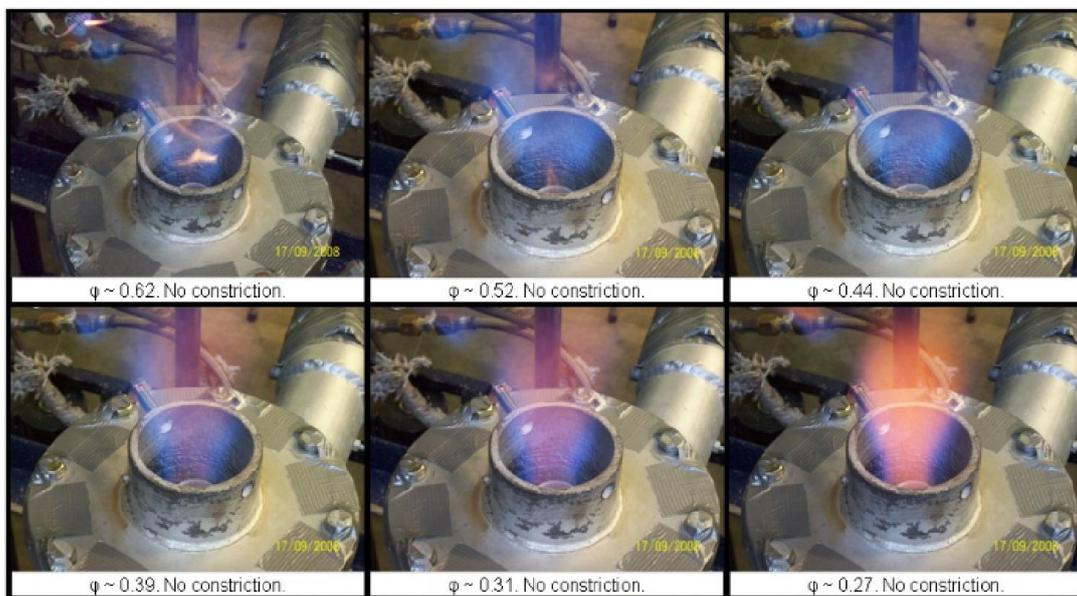
Figure 10. Non-constricted exhaust case at different equivalence ratios. Gas Injection of 25 l/min diffusive (Wide Injector), 40 l/min premixed
