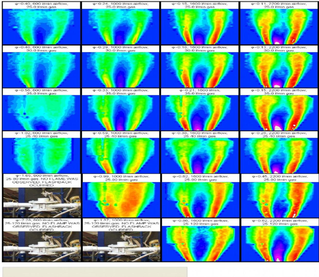
Figure 9. Fixed air flow rates, different modes of gas injection and gas rates. Wide Injector Used. Colour bar in (m/s). Initial CRZ formation after Vortex breakdown occurs as a wobbling unattached weak (blue) region, very difficult to visualize. The CRZ is completely attached to the fuel injector, very coherent and strong (purple), being very easy to follow for visualization purposes
