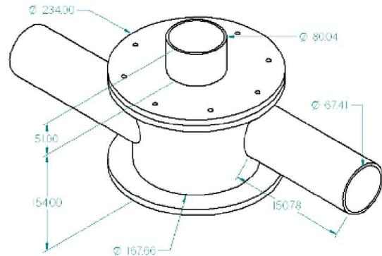
Figure 1. Swirl Burner geometry in Unconfined mode (mm)
