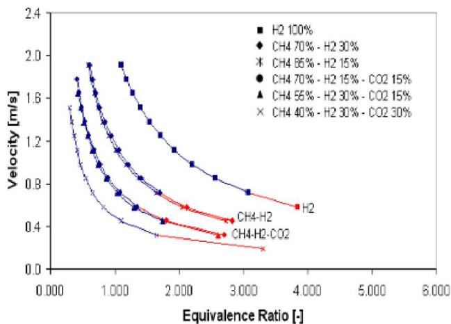
**Figure 21. Flashback analysis for different blends at 1400l/min air flow using No Exhaust Nozzle Constriction at 5-40 l/min gas injection. Flashback (red) and nonflashback conditions (blue). CH4-H2 blends have almost the same trend, as well as CH4-H2-CO2 at 15% CO2**
