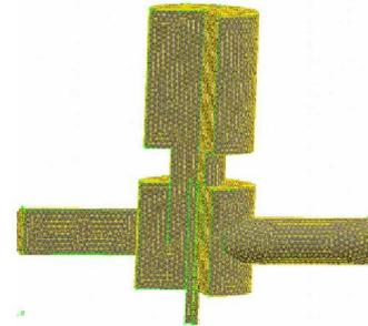
Figure 4. Tangential Swirl Burner Model
