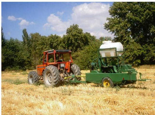
Figure 2. Cereal Straw Urea Treatment Machine (CSUTM)
