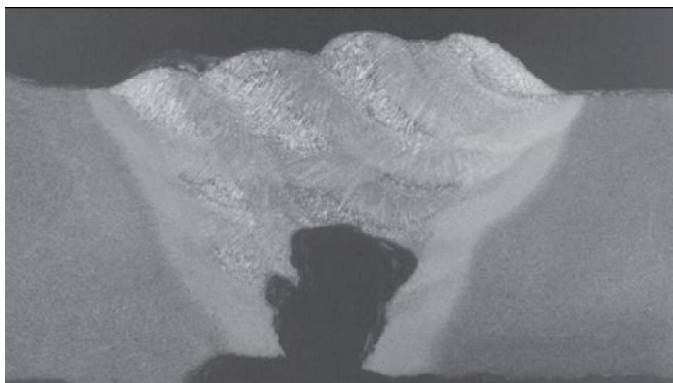
Fig. 4. Carbon Steel Weld Root Corrosion (Photo courtesy ESR Tech.) 3
