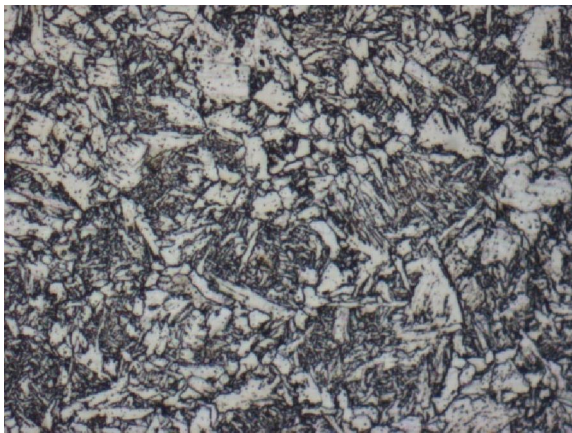
Fig.7b.Electrode 8018G-Weld microstructure (Coarse columnar- 200x)
