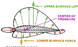
CAMBERED AIRFOIL AT POSITIVE LIFT
