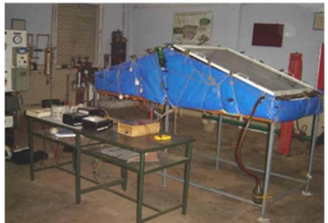
Figure 3. Experimental setup of still-solar
