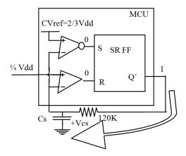
Fig. 11. Oscillator operation
