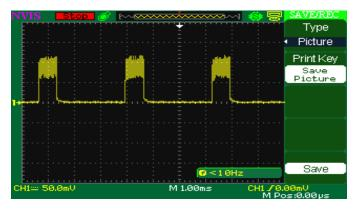
Fig. 24 Signal at port.0 in mode 0 from slider board after touch event
