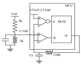
Fig. 9. Relaxation oscillator circuit
