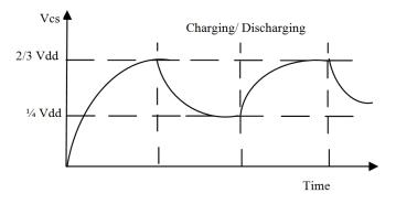
Fig. 15. Vcs voltage Charging & discharging waveform
