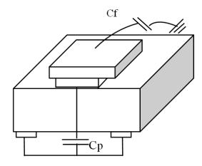
Fig. 4. Capacitance generated in touch screen sensor after occurring touch event
