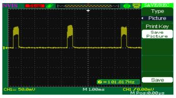
Fig. 22. Signal waveform from Matrix board at Port.8 before touch
