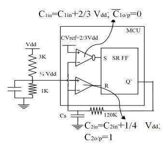
Fig. 8. Relaxation oscillator circuit
