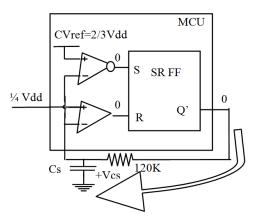
Fig. 13. Oscillator operation
