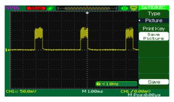
Fig. 21. Signal waveform at port.8 when key 8 at touch occurs
