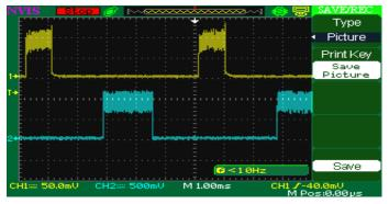
Fig. 23. Signal at port.8 & .1 when key 0 on Matrix board touched
