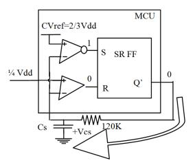
Fig. 12. Oscillator operation
