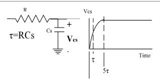
Fig. 6. Touch screen output signal before touch event
