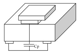
Fig. 3. Capacitance before touch
