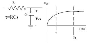
Fig. 7. Touch screen output signal after touch event
