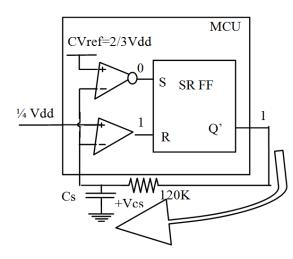
Fig. 14. Oscillator operation
