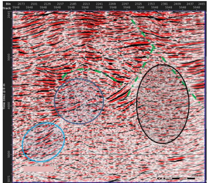
Fig. 5. 3d PSDM section after detailed velocity analysis as applied in this study; event continuity is enhanced within the circled zones; Fault lines are clearer and a rollover structure becomes more identifiable than in the previous section
