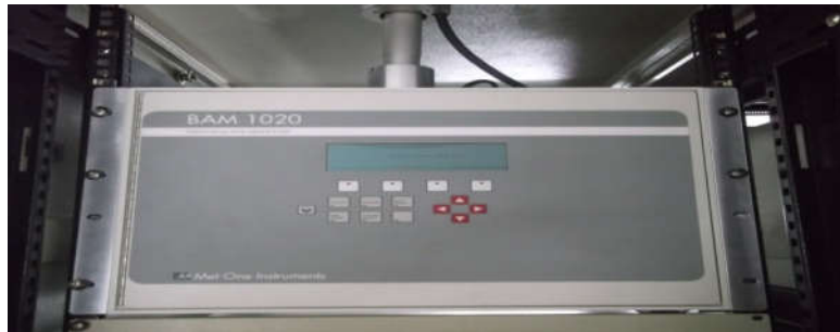
Figure (2) - BAM (Beta Attenuation Monitor) Instrument
