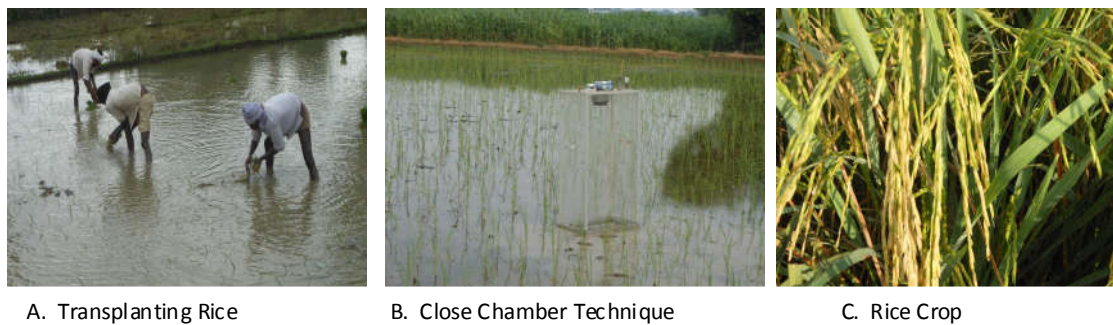
Fig.2. Close chamber technique employed in rice fields for CH_4 and N_2O gases sampling
