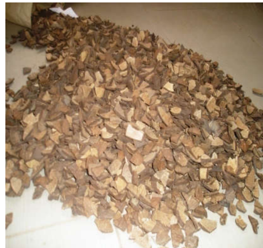
Plate II. Machine crushed Coconut shell aggregate
