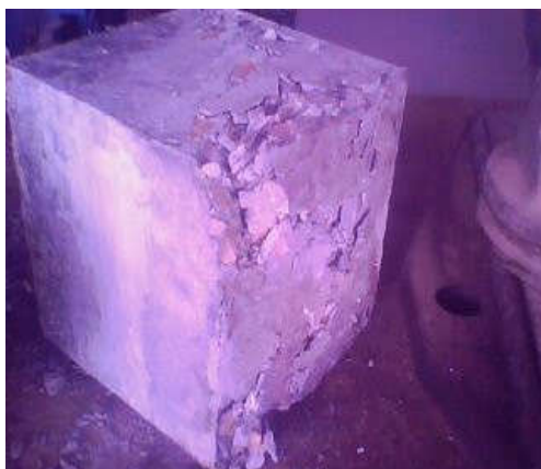
Plate VII: Showing Coconut shell concrete cube for mix ratio 1:1:1 after test 28 day. Plate VIII: Showing the cube produced for mix ratio 1:2:2
