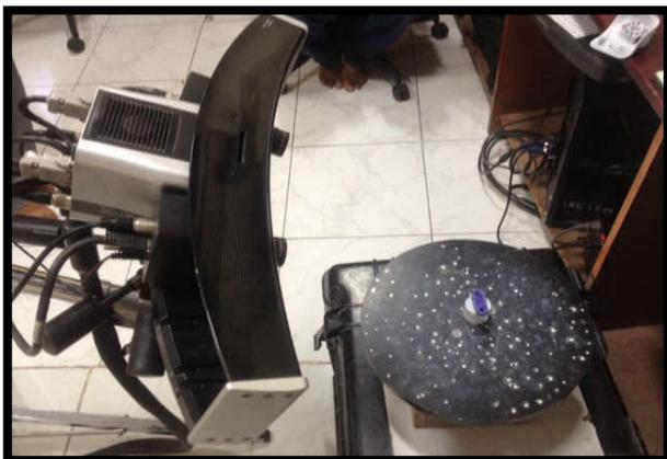
Fig.7. 3D scanner (Solnix, Rexscan-3, Germany)
