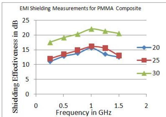
Fig. 11. EMI Measurements for PMMA Composite sheet for 30% Ni-P-W CNC
