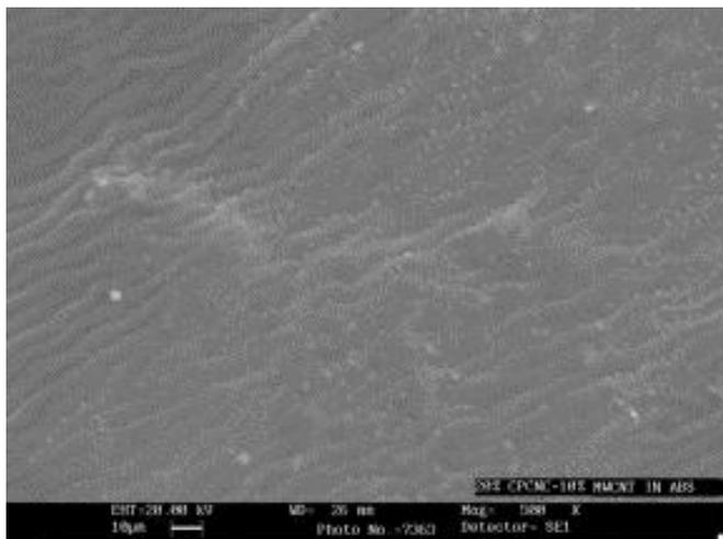
Fig.9. SEM micrograph of ABS composite sheet at 500X (30% Ni-P-W CNC)
