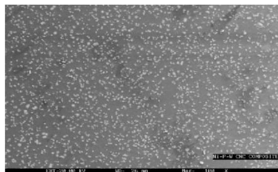
Fig. 7. SEM micrograph of ABS composite sheet at 100X (25% Ni-P-W CNC)
