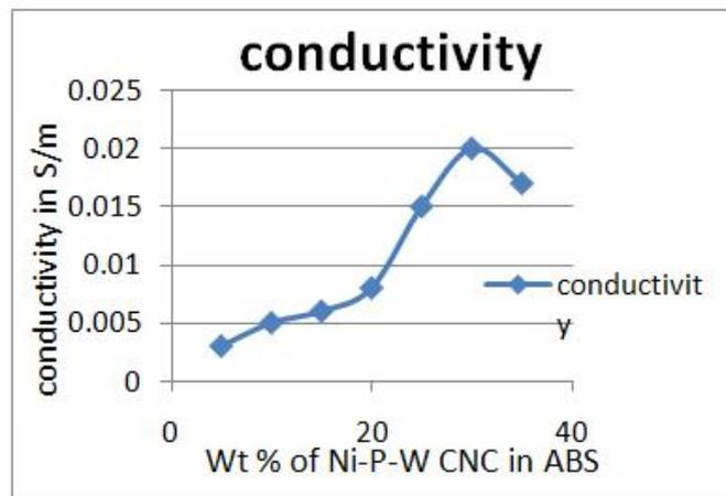
Fig. 12. Conductivity of ABS composite sheet for different wt% of Ni-P-W CNC
