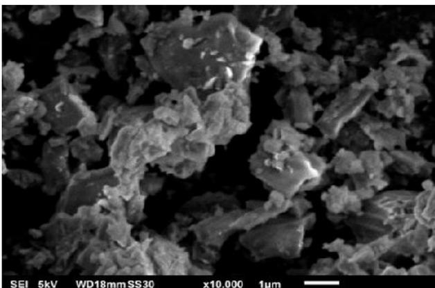
Fig. 5. SEM micrograph of Ni-P-W CNC at 10KX
