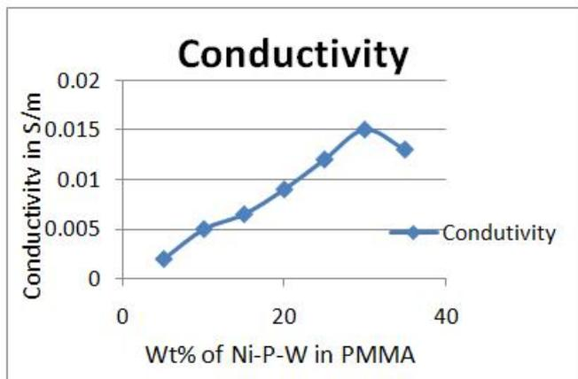
Fig. 10. Conductivity of PMMA composite sheet for different wt% of Ni-P-W CNC
