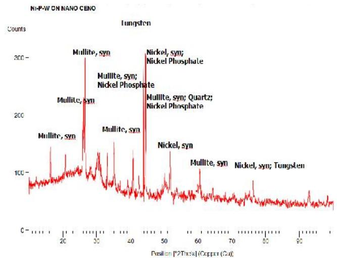
Fig. 1. XRD of Ni-P-W CNC
