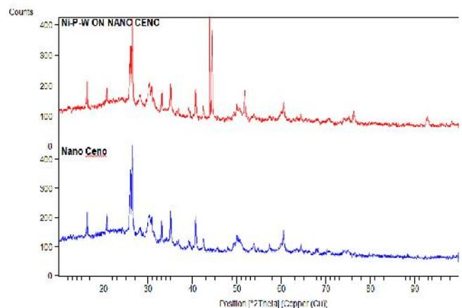
Fig. 2. Comparison of XRD of NC and Ni-P-W CNC
