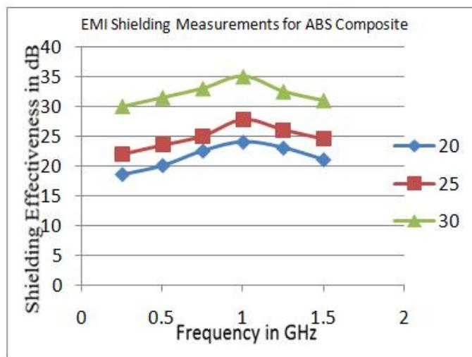
Fig. 13. EMI Measurements for ABS Composite sheet for 30% Ni-P-W CNC
