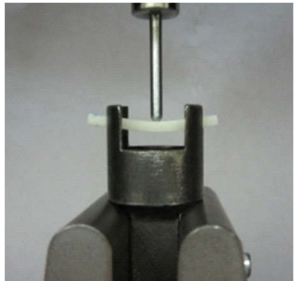
Fig.3. Flexural strength specimen under load in UTM
