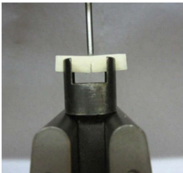
Fig.6. Fracture resistance specimen under load in UTM
