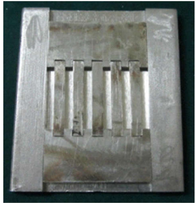
Fig.1. Master die for fabrication of flexural strength test specimens
