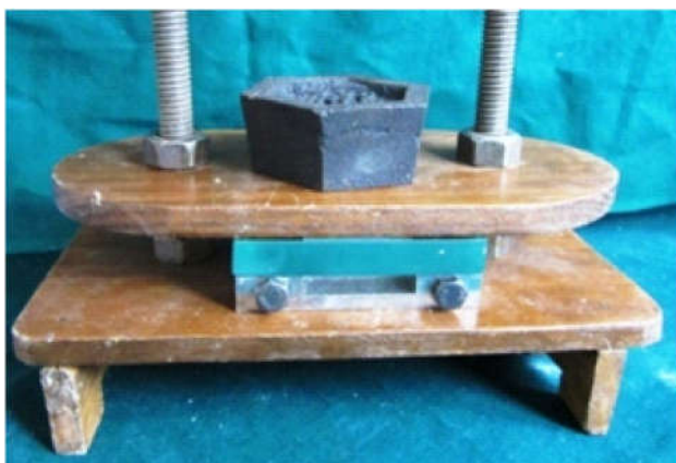
Fig.5. Load application during setting of fracture resistance test specimens
