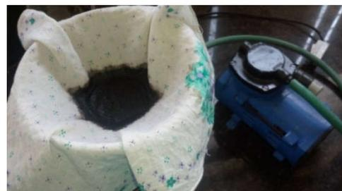
Fig.5. Washing of carbonized powder
