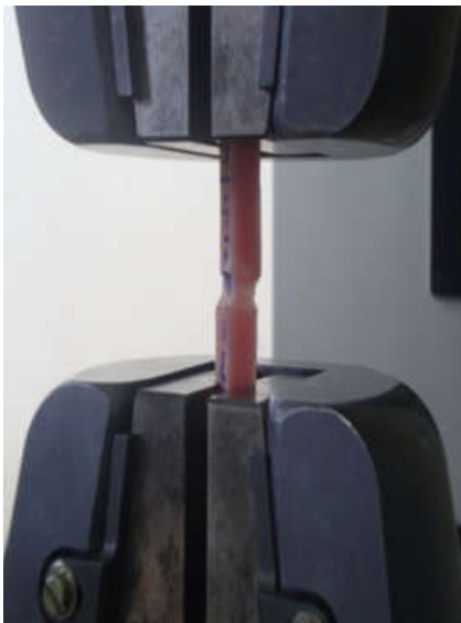
Fig. 4. Tensile bond strength measurement using universal testing machine
