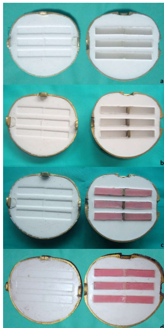
Fig. 2. Sample showing resilient denture liner sandwiched between two heat polymerized denture base resin blocks
