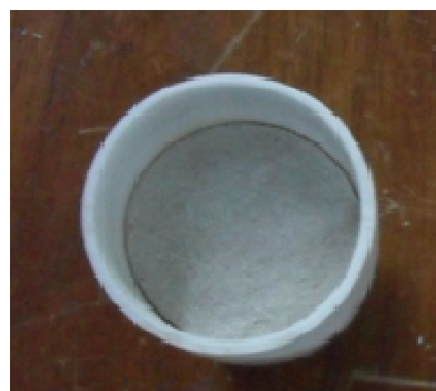
Figure 5. Changes in color of combustions residues after calcination on a laboratory furnace
