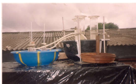
Fig. 1. Digestor set-up for biogas production of the wastes
