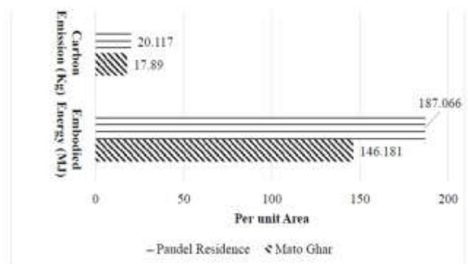
Figure 11. Comparative Study of calculation of Embodied Energy and Carbon Emission of Mato Ghar & Paudel Residence
