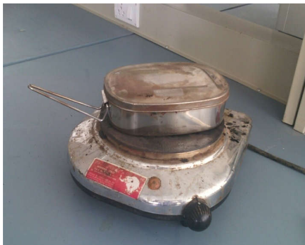
Figure 7. Melting point determination of plastic waste with and without catalyst
