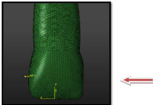
Fig 5. Tipping -60 gms of force directed in the horizontal direction, perpendicular to the long axis of the tooth
