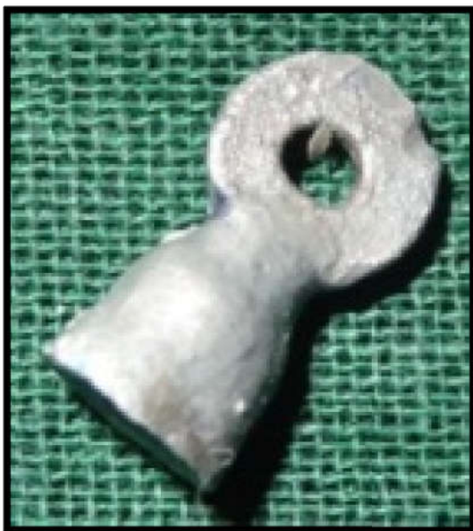
Figure 1.8. Casted coping with Co-Cr alloy
