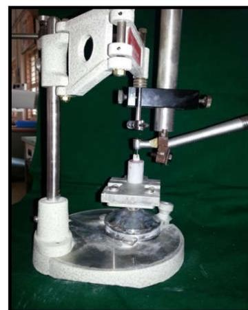
Figure 3. Bur parallel to vertical rod
