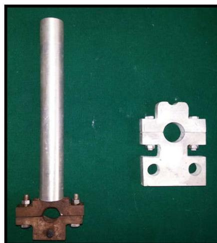
Figure 2. Jig for standardizing tooth preparation
