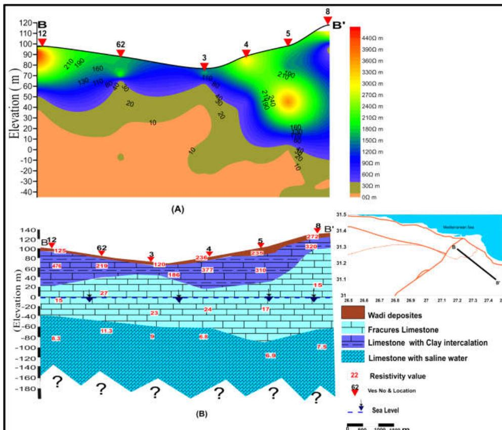
Figure 12. Geoelectrical Cross Section BB'
