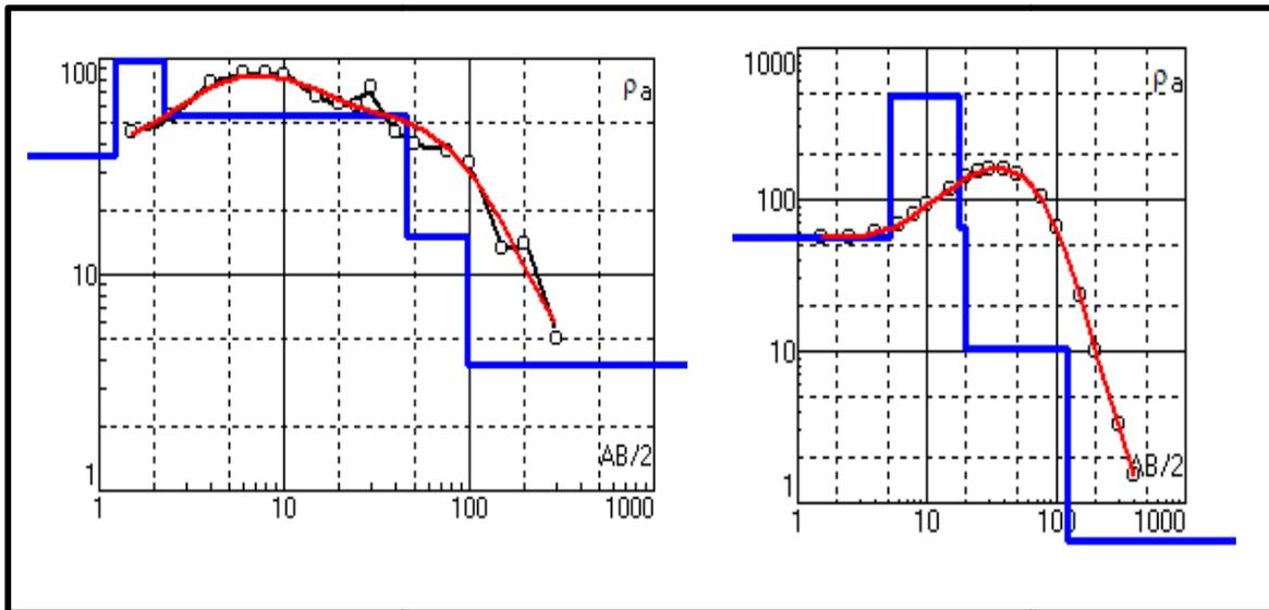
Figure 6. Interpreted Field Curves Data for VES, s(4 and 6)
