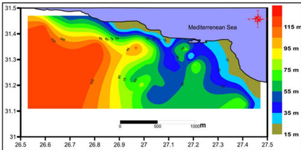
Figure 8. Contour Map of the Depth to the Upper Part of the Aquifer
