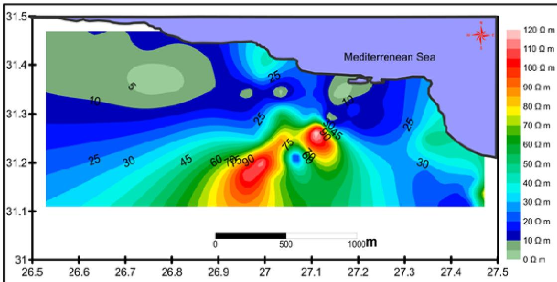
Figure 9. True Resistivity Contour Map of Fracture Limestone Layer
