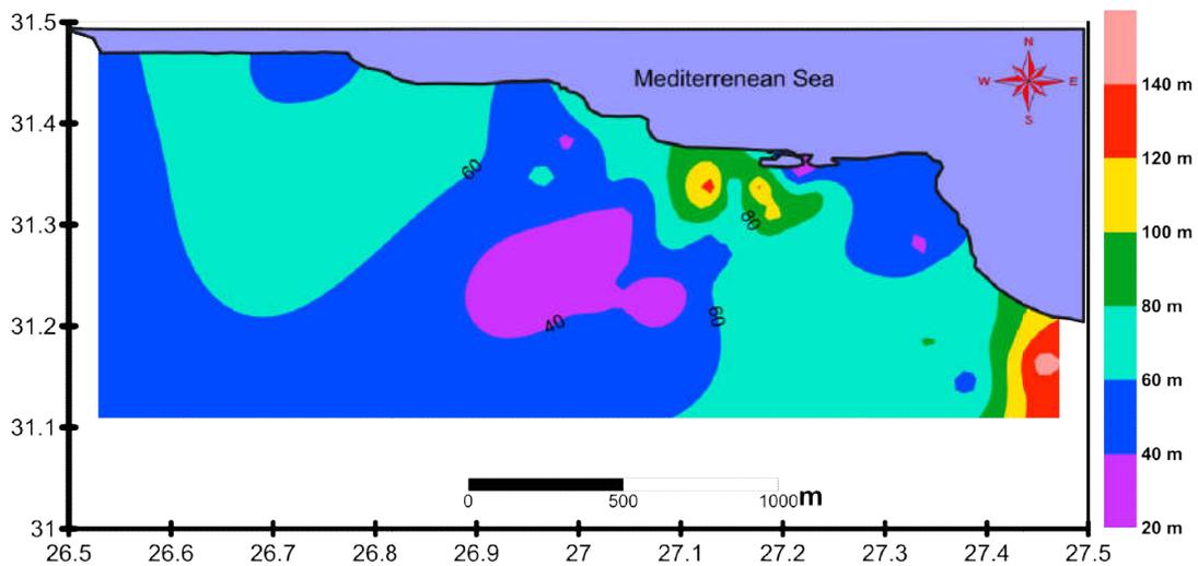
Figure 7. Isopach Contour Map of the Upper Part of the Aquifer
