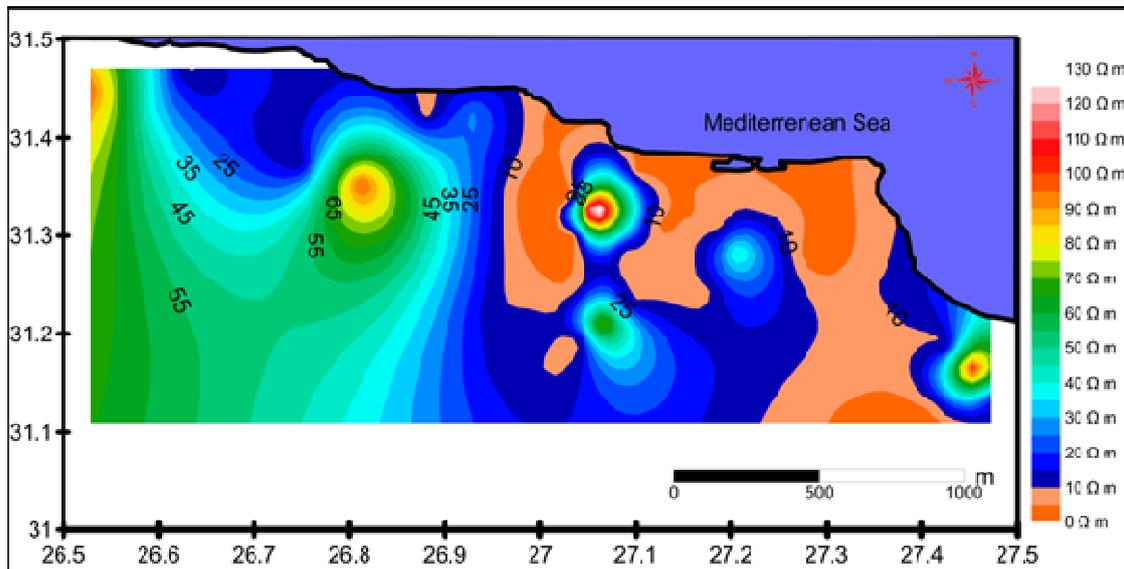
Figure 10. True Resistivity Contour Map of Fourth Layer
