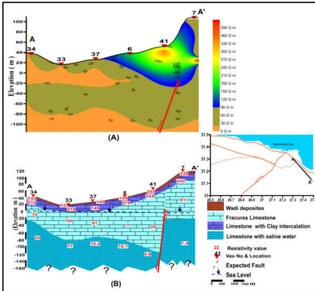
Figure 11. Geoelectric Cross-Section A-A
