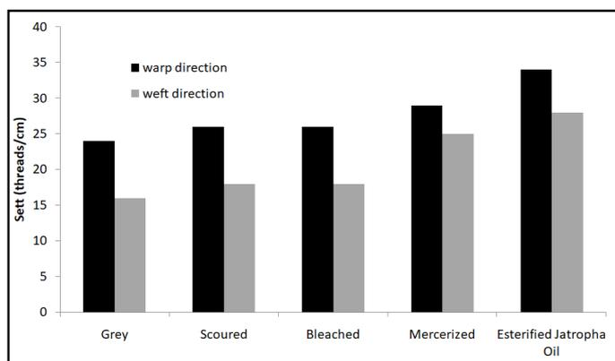
Figure 3. Effect of treatments on fabric sett (Warp and Weft Directions)
