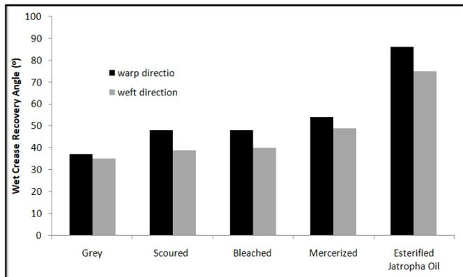
**Figure 6. Effect of treatments on wet crease recovery angle (Warp and Weft Directions)**
