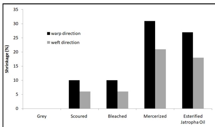
Figure 4. Effect of treatments on fabric shrinkage (Warp and Weft Directions)
