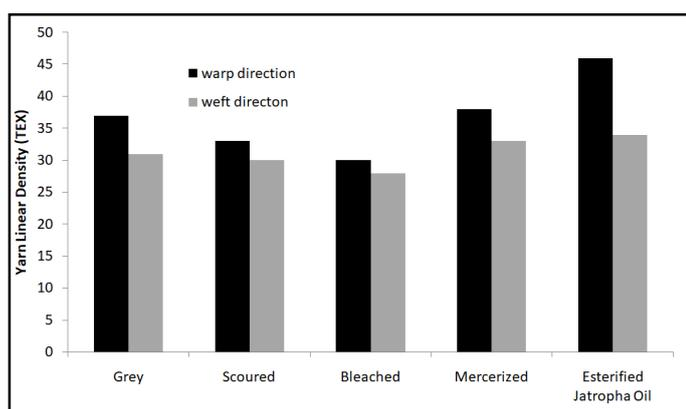
Figure 2. Effect of Treatments on yarn linear density (Warp and Weft Directions)
