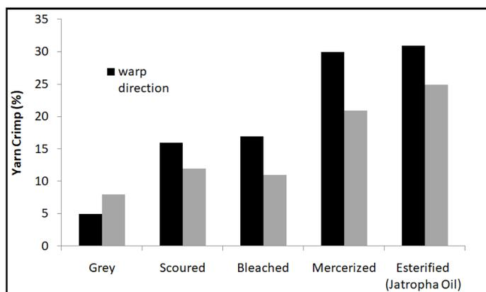
Figure 1. Effect of treatments on yarn crimp (Warp and Weft directions)
