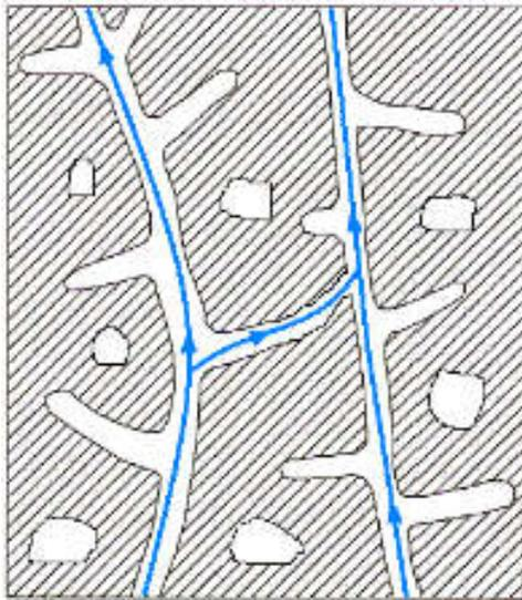
Fig. 1. Diagram of liquid flow through a porous deposit rigid frame-structured channel with open flow channels and blind and closed pores (Szmigielski, 2006)
