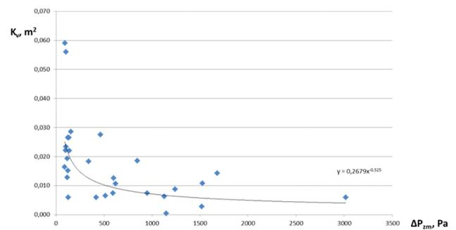
Fig. 6. Effect of flow resistance  $\Delta P_{zm}$  on the gas permeability coefficient  $K_V$  of the adhesive bed - - distribution of experimental points.
