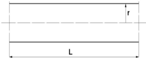
Fig. 2. Burdine's cylindrical capillary model (Burdine, 1953): L - length, r - radius
