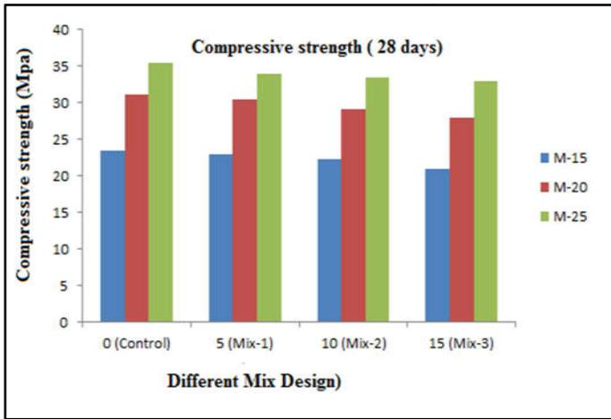
**Figure 2. Compressive strength of 28 Days (Different Mixes)**
