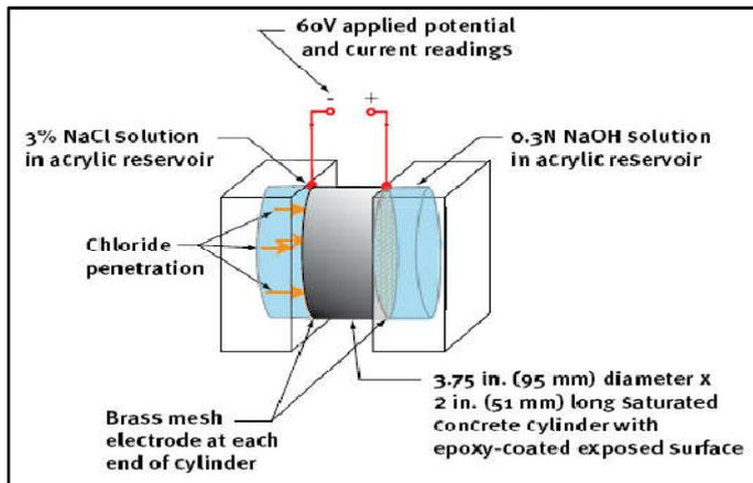
Figure 6. Rapid Chloride Ion Permeability Apparatus
