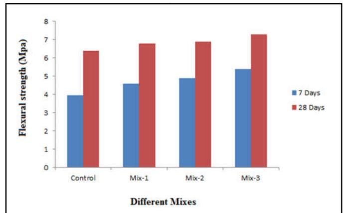
**Figure 4. Flexural strength of different Mixes**
