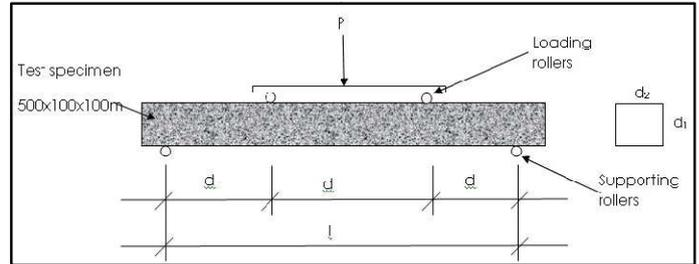
**Figure 3. Set up for Flexural strength test**
