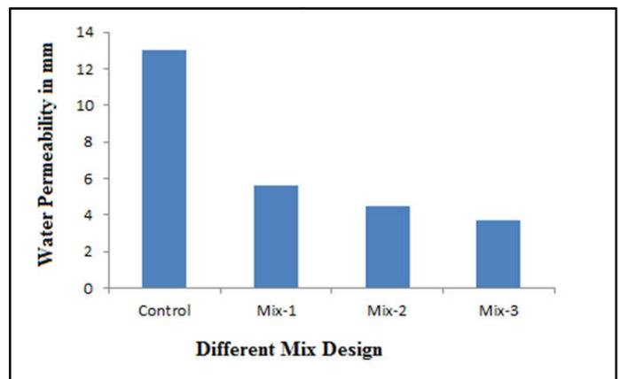
**Figure 5. Water permeability of different mixes**
