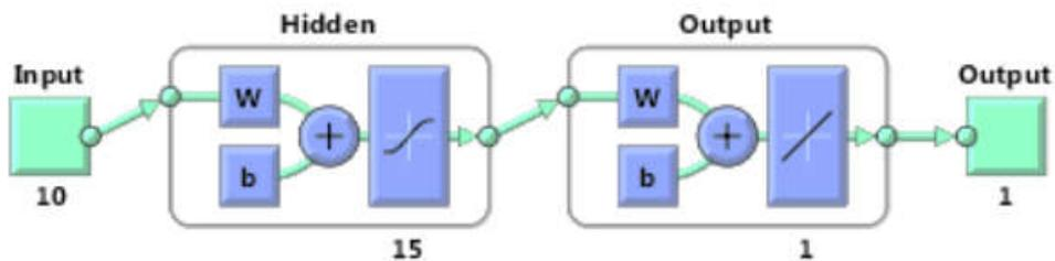
Figure 4. Internal structure of the developed three-layer back propagation neural networks
