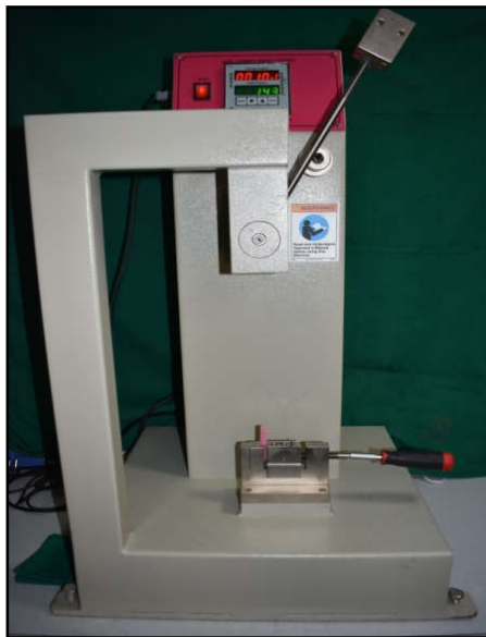
Fig. 4. Izod impact testing machine with specimen in position
