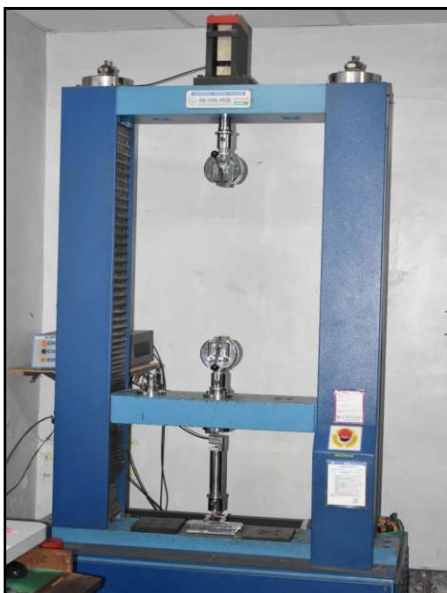
Fig. 5. Universal testing machine with specimen in position
