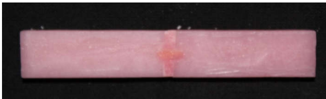
Fig. 3. Aramid fiber reinforced repaired sample
