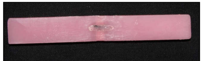
Fig. 2. Carbon fiber reinforced repaired sample
