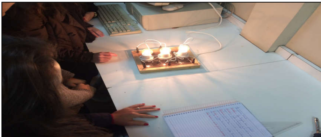
Figure 10. Connecting Lamps in Series and Parallel
