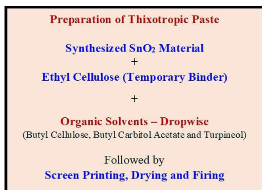
Fig. 3. Thick film fabrication route
