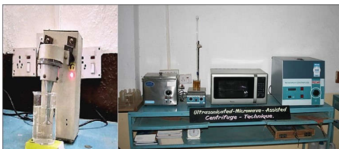
Fig. 1 (a): Disc type ultrasonicator Fig. 1 (b): Microwave treatment followed centrifuge technique
