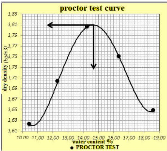
Figure 3. Proctor test curve
