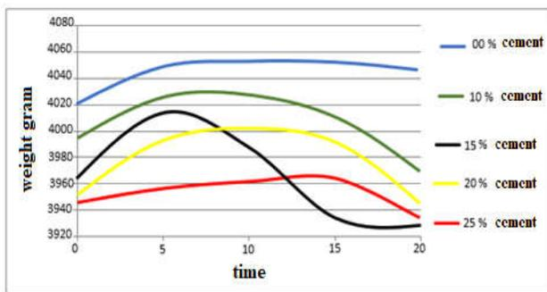
Figure 4. Curves of water absorption by cement stabilized bricks as a function of time
