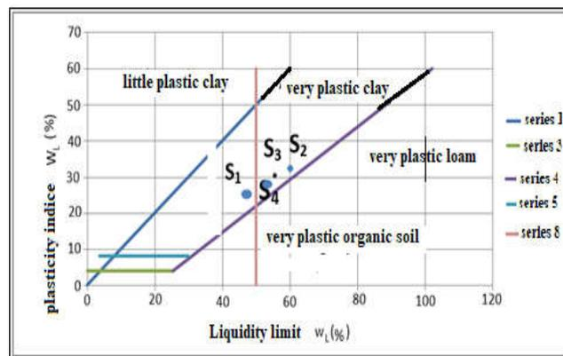
**Figure 2. Casagrande diagram**
