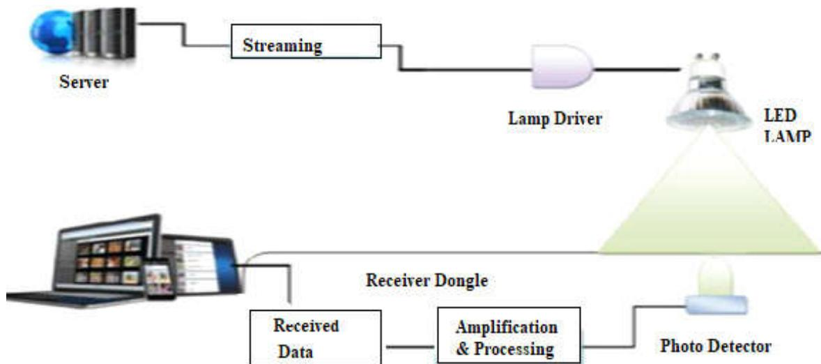
Figure 1. Showing basic structure of LI-FI system
