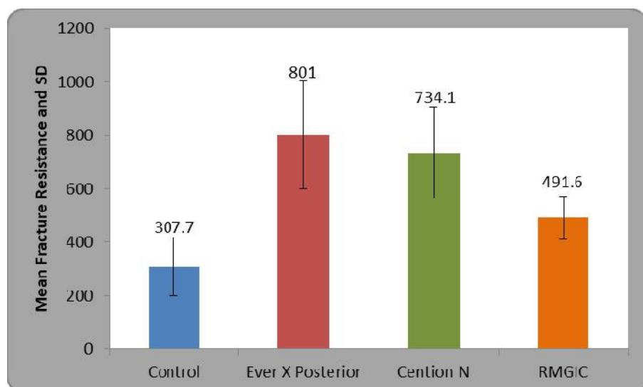
By using one way ANOVA statistically significant variation was found in mean fracture resistance in samples of four groups ( $F=23.37, p=0.0001$ ).
