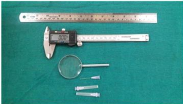
Photograph 2: Scale, Digital calliper, Hand lens, Hypodermic needle (24 gauge)
