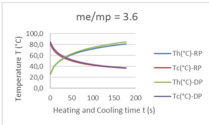
Figure 10-d. Plaster samples heating and cooling thermograms  $\frac{m_e}{m_p} = 3.6$
