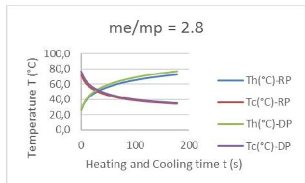
Figure 10-c. Plaster samples heating and cooling thermograms  $\frac{m_e}{m_p} = 2.8$
