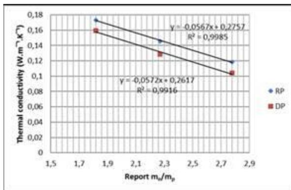
Figure 8. Eco-plaster thermal conductivity according to mixing rate
