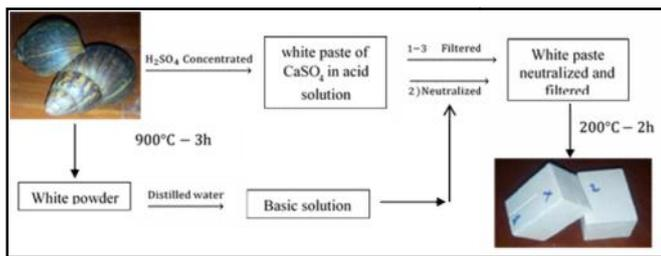
Figure 2. Eco-plaster synthesis from snail shells
