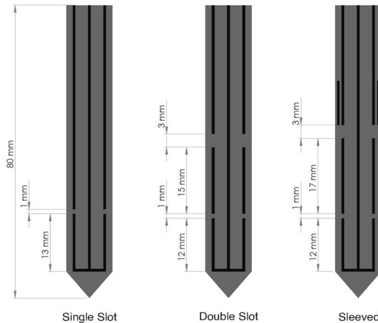
Fig. 1. Model geometry of single slot, double slot and sleeved antennas
