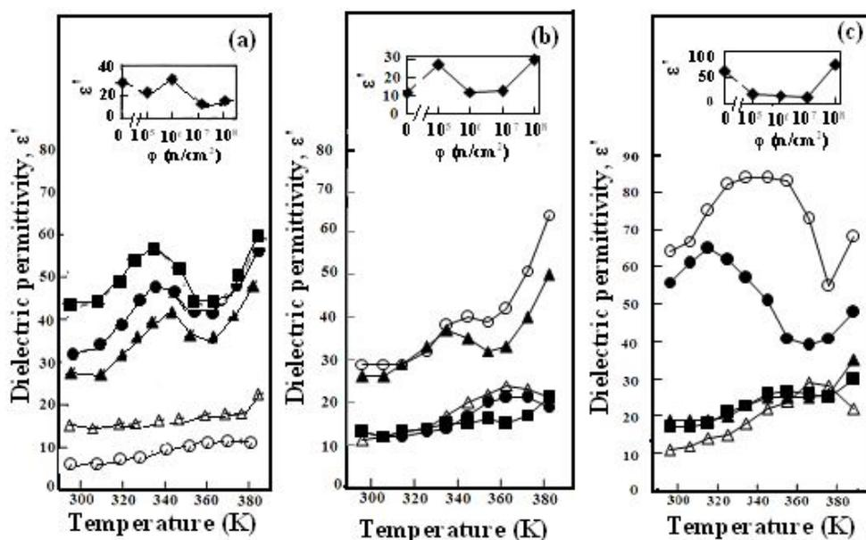
Figure 3: Temperature dependence of the dielectric permittivity ( $\epsilon'$ ) for unirradiated and irradiated 100/0 (a), 92/8 (b) and 88/12 wt/wt% (c), PVA/HPC blended samples with different fast neutron fluencies at 10 kHz: (●) unirradiated, (▲)  $1 \times 10^5$ , (■)  $1 \times 10^6$ , (△)  $1 \times 10^7$  and (○)  $1 \times 10^8$  n/cm<sup>2</sup>. The inset of the figure shows the variation of  $\epsilon'$  as a function of neutron fluencies ( $\phi$ ) at 10 kHz and 310 K.
