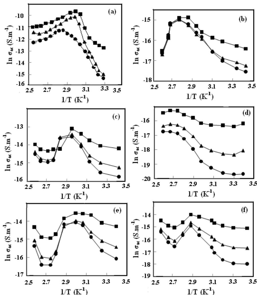
Figure 7: Reciprocal temperature dependence of the a.c. conductivity ( $\ln \sigma_{ac}$ ) for PVA/HPC blended samples at different frequencies: (a) 100/0, (b) 0/100, (c) 96/4, (d) 92/8, (e) 88/12 and (f) 84/16 wt/wt%. (●) 1 kHz, (▲) 10 kHz and (■) 100 kHz.
