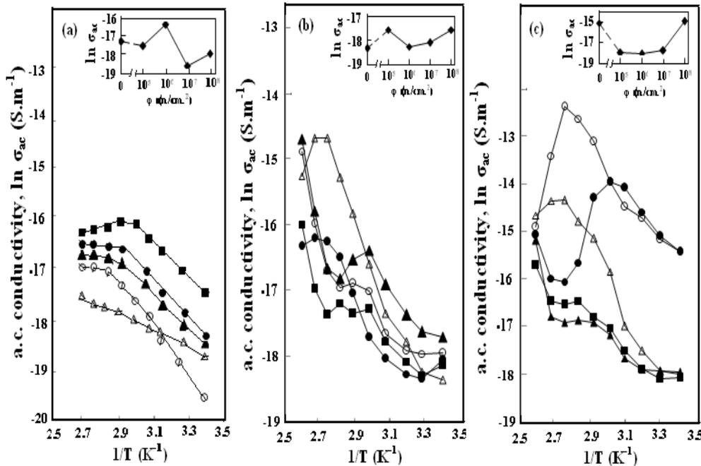
Figure 9: Reciprocal temperature dependence of the a.c. conductivity ( $\ln \sigma_{ac}$ ) for unirradiated and irradiated 100/0 (a), 92/8 (b) and 88/12 wt/wt% (c), blended samples with different fast neutron fluencies at 10 kHz: (●) unirradiated, (▲)  $1 \times 10^5$ , (■)  $1 \times 10^6$ , (△)  $1 \times 10^7$  and (○)  $1 \times 10^8$  n/cm<sup>2</sup>. The inset of the figure shows the variation of  $\ln \sigma_{ac}$  as a function of neutron fluencies ( $\phi$ ) at 10 kHz and 310 K.
