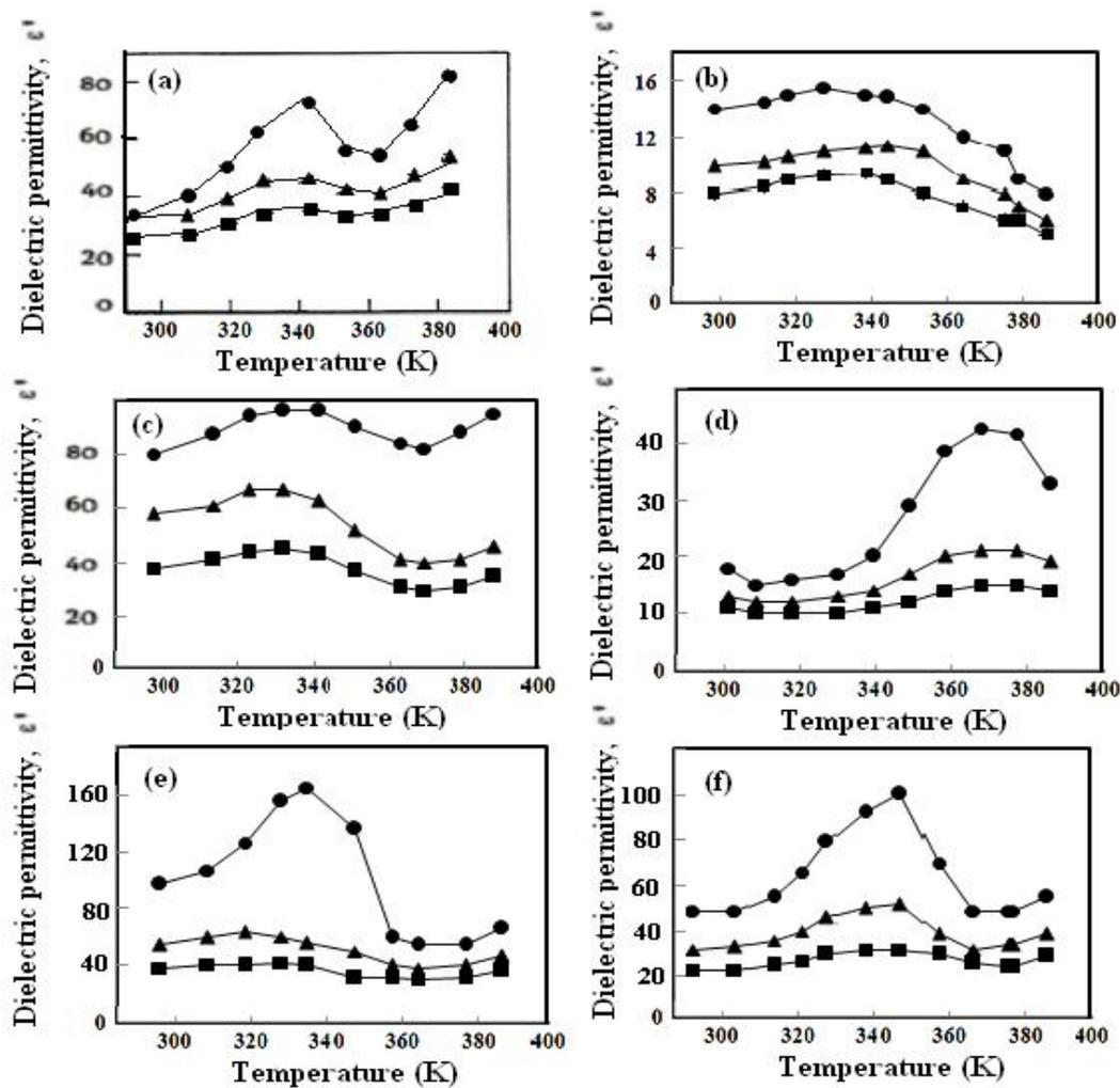
Figure 1: Dependence of dielectric permittivity ( $\epsilon'$ ) on temperature at different frequencies for PVA/HPC blended samples: (a) 100/0, (b) 0/100, (c) 96/4, (d) 92/8, (e) 88/12 and (f) 84/16 wt/wt%. (●) 1 kHz, (▲) 10 kHz and (■) 100 kHz.
