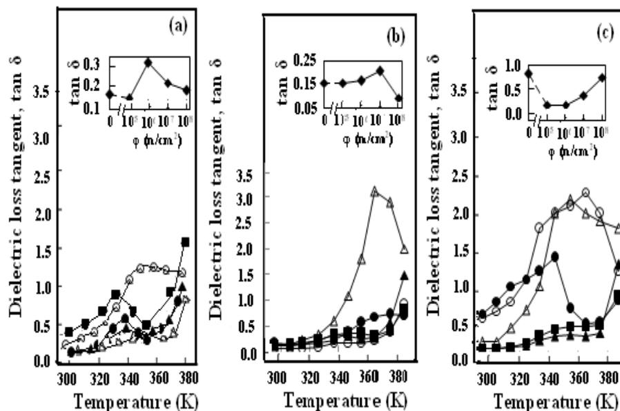
Figure 6: Temperature dependence of the dielectric loss tangent ( $\tan \delta$ ) for unirradiated and irradiated 100/0 (a), 92/8 (b) and 88/12 wt/wt% (c), PVA/HPC blended samples with different fast neutron fluencies at 10 kHz: (●) unirradiated, (▲)  $1 \times 10^5$ , (■)  $1 \times 10^6$ , (△)  $1 \times 10^7$  and (○)  $1 \times 10^8$  n/cm<sup>2</sup>. The inset of the figure shows the variation of  $\tan \delta$  as a function of neutron fluencies ( $\phi$ ) at 10 kHz and 310 K.
