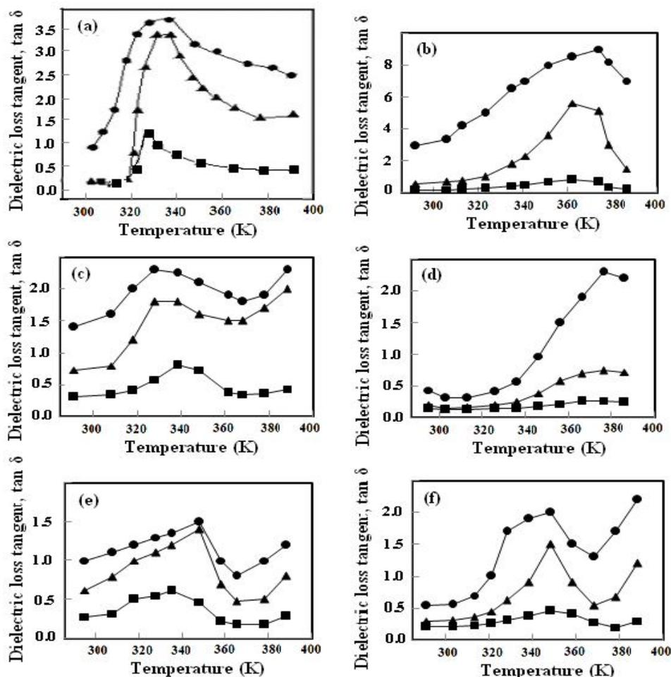
**Figure 4:** Dependence of the dielectric loss tangent ( $\tan \delta$ ) on temperature at different frequencies for PVA/HPC blended samples: (a) 100/0, (b) 0/100, (c) 92/8 and (d) 88/12 wt/wt%. (●) 1 kHz, (▲) 10 kHz and (■) 100 kHz.
