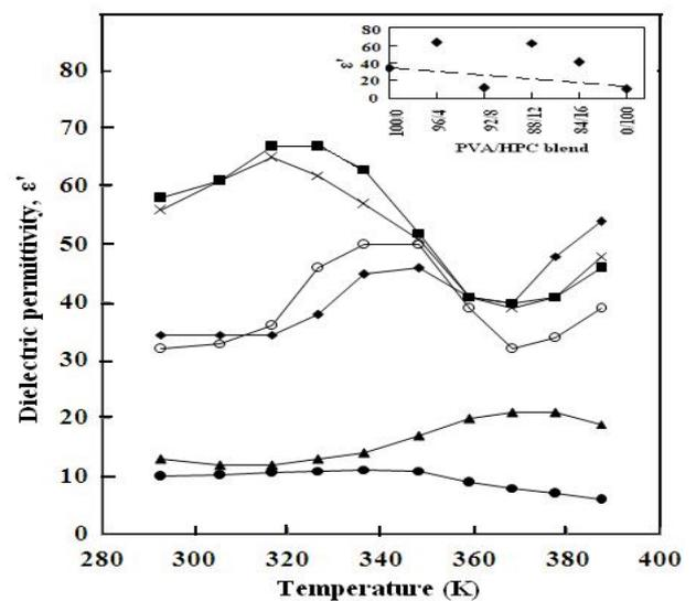
Figure 2: Temperature dependence of the dielectric permittivity ( $\epsilon'$ ) for PVA/HPC blended samples at 10 kHz: (●) 100/0, (■) 96/4, (▲) 92/8, (x) 88/12, (◊) 84/16 and (○) 0/100 wt/wt%. The inset of the figure shows the variation of  $\epsilon'$  as a function of HPC concentration at 10 kHz and 310 K.
