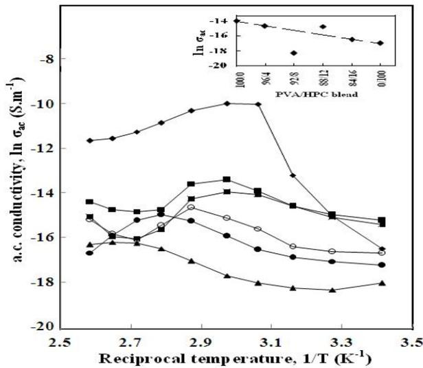
Figure 8: Reciprocal temperature (1/T) dependence of the a.c. conductivity ( $\ln \sigma_{ac}$ ) for PVA/HPC blended samples at 10 kHz: (♦) 100/0, (■) 96/4, (▲) 92/8, (x) 88/12, (o) 84/16 and (●) 0/100 wt/wt%. The inset of the figure shows the variation of  $\ln \sigma_{ac}$  as a function of HPC concentration at 10 kHz and 310 K.
