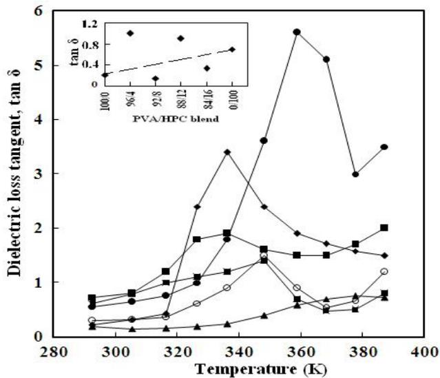
Figure 5: Temperature dependence of the dielectric loss tangent ( $\tan \delta$ ) for PVA/HPC blended samples at 10 kHz: (♦) 100/0, (■) 96/4, (▲) 92/8, (○) 88/12, (□) 84/16 and (●) 0/100 wt/wt%. The inset of the figure shows the variation of  $\tan \delta$  as a function of HPC concentration at 10 kHz and 310 K.
