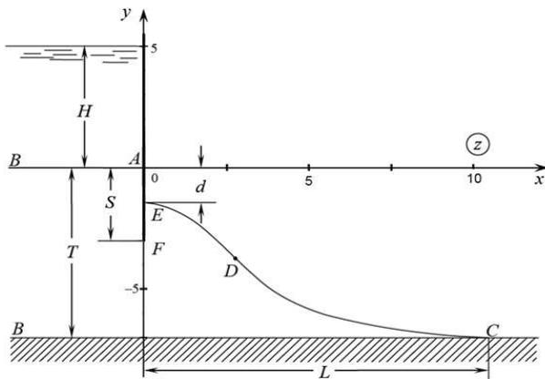
Fig. 1. 6. The current picture calculated at  $\epsilon = 0.6$ ,  $T = 7$ ,  $S = 3$ ,  $H = 7$ ,  $H_0 = 3$ ,  $h_c = 100$
