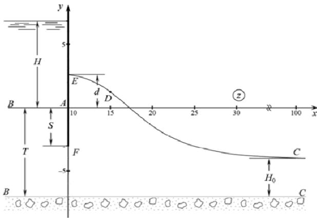
Fig. 1. a. The current picture calculated at  $\epsilon = 0.6$ ,  $h_c = 0.5$ ,  $T = 7$ ,  $S = 3$ ,  $H = 5$ .
