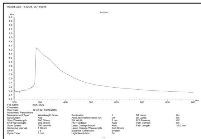
**Fig. 3(b).** UV-Vis spectrum of aqueous medium during biosynthesis of copper nanoparticles using *O. tenuiflorum*
