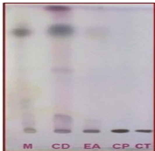
Figure e. Comparatives TLC of ethanolic extracts of CD, CT, EA and CP with mangiferin (M) (Rf: 0.72 with 1% FeCl 3 sol)
