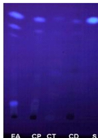
Figure d: Comparatives TLC of ethanolic extracts of CD, CT, EA and CP with scopolatin (S) (Rf= 0.81 in UV 366 nm.)
