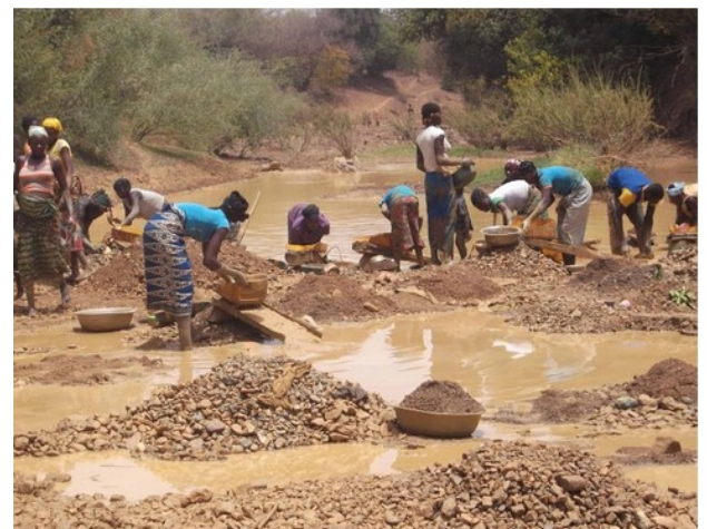
Figure 4. Soil degradation by small scale gold mining
