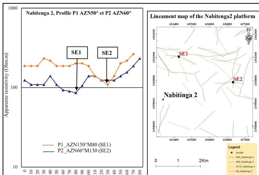
Figure 10. The electrical resistivity curves on the Nabitenga2 platform
