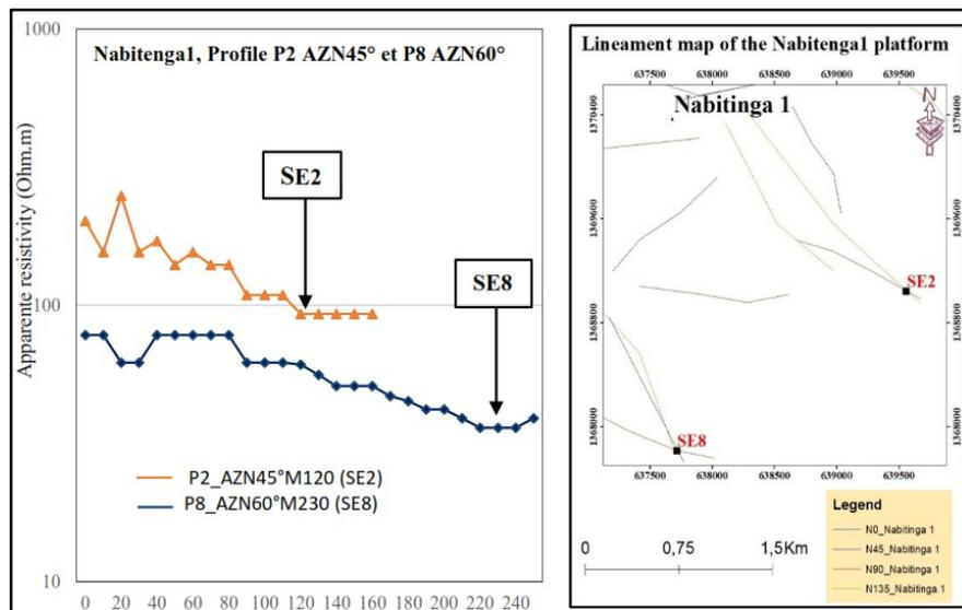
Figure 9. The electrical resistivity curves on the Nabitenga1 platform.
