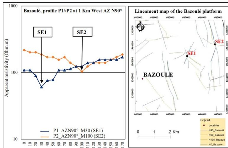
Figure 6. Electrical resistivity profiles on the Bazoulé platform
