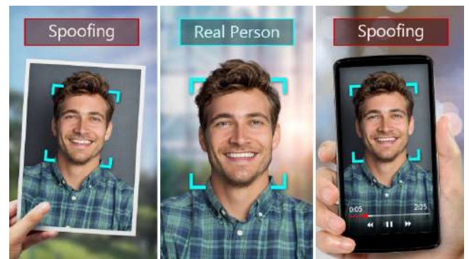
Fig. 10. Comparison of Vitality Detection of Photo Graphic Image and Mobile Image with Live Person
